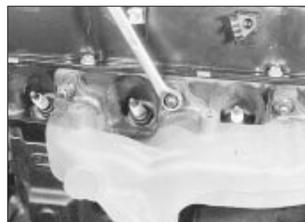
26.6a Unscrew the exhaust manifold securing nuts . . .
