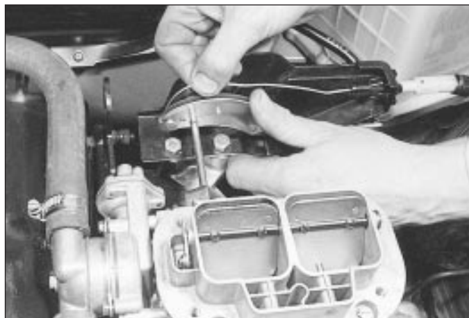
12.6 Disconnecting the throttle cable end from the throttle lever - Weber 2V carburettor
