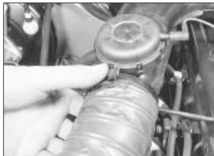
3.3 Disconnecting the cold air intake hose from the air cleaner spout
