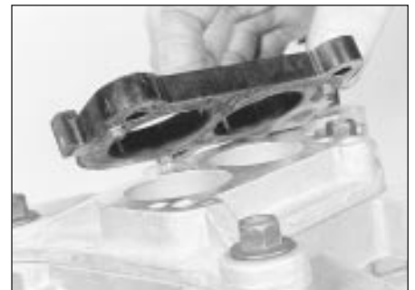
25.49b . . . and the insulator block from the inlet manifold - CVH models
