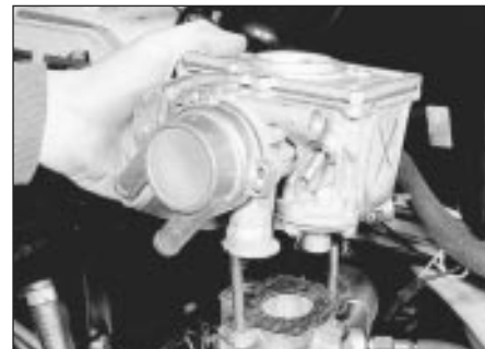
14.8b . . . and lift the carburettor from the inlet manifold - Ford VV carburettor
