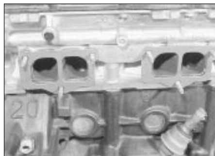
26.8a Exhaust manifold gaskets in position on cylinder head - DOHC models
