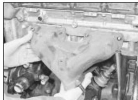
26.8c Fitting the exhaust manifold - DOHC models
