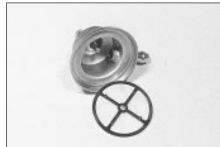
8.7 Removing the top cover from an early type fuel pump for access to the mesh filter
