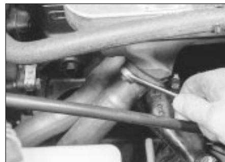
26.4 Unscrewing an exhaust downpipe securing nut
