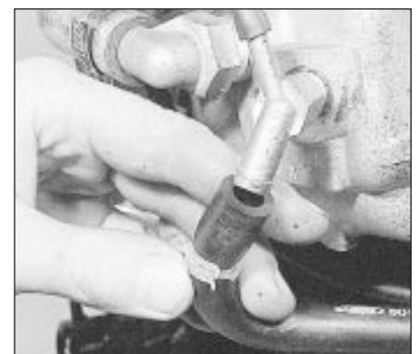
25.8a Disconnecting the crankcase ventilation . . .
