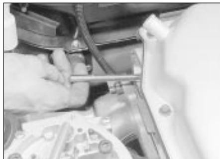
8.5 Withdrawing the fuel pump operating pushrod - CVH model
