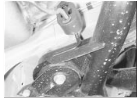
27.5a Rear exhaust section mounting - Hatchback model
