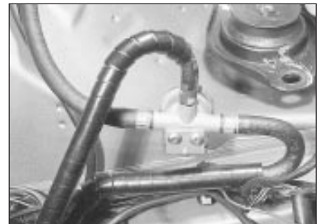
5.1 Fuel pressure regulator location - models up to 1985
